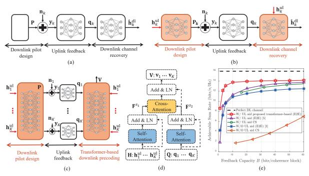
Figure 1 (a) The E2E scheme for downlink channel estimation without uplink aid [3], (b) the E2E scheme for downlink channel estimation with uplink aid [5], (c) the proposed transformer-based E2E scheme for downlink precoding with uplink aid, (d) the proposed transformer-based precoding model, and (e) the comparison of achievable sum rate performance.
